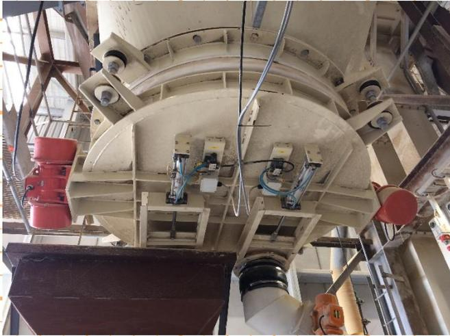
Unique in that multiple outlets can be fitted, each having variable feed rates and capable of individual operation. Vibratory action provides constant performance under changing head load.
