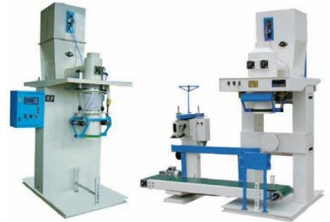
The Weighing and Bagging Machine is a combined weighing and bagging system to serve the bagging operations of powdery materials. It includes a high capacity bagging scale, feeder, bagging table, bag shaker, sewing line and transfer conveyer
