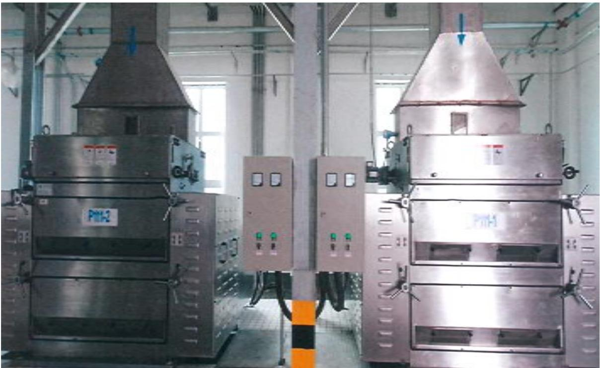
Two high capacity flaking roller mills installed within soya bean flaking arrangement.
