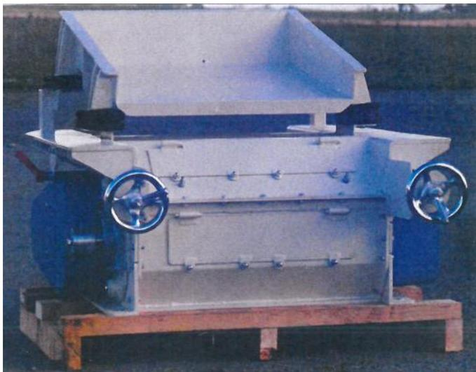
Different feeder types are supplied to suit the product being handled including roll feeders, pin feeders and vibratory tray type feeders. Adjustment is made to the product feed rate through alteration of the feed roll or tray speed or amplitude in combination with regulation of the adjustable feed gate.
