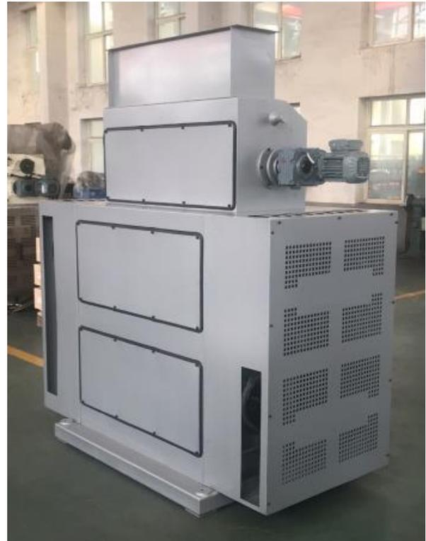
5. Two high roller mill complete with two pair of 1000mm L x 300mm diameter fluted rolls for general purpose grain crimping and grinding application.
