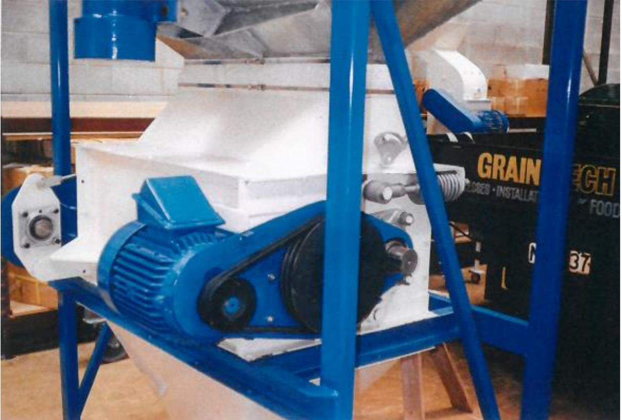
5. Feeders may be of either the roll feeder, pin feeder or vibratory feeder type and each is fitted to be fully adjustable and with a controlled feed gate. A variable speed control drive may be incorporated where required for adjusting the feed rate for a wide variety of products to be processed. A by-pass gate can be fitted into the roller mill to enable product to be diverted past the grinding rolls.
