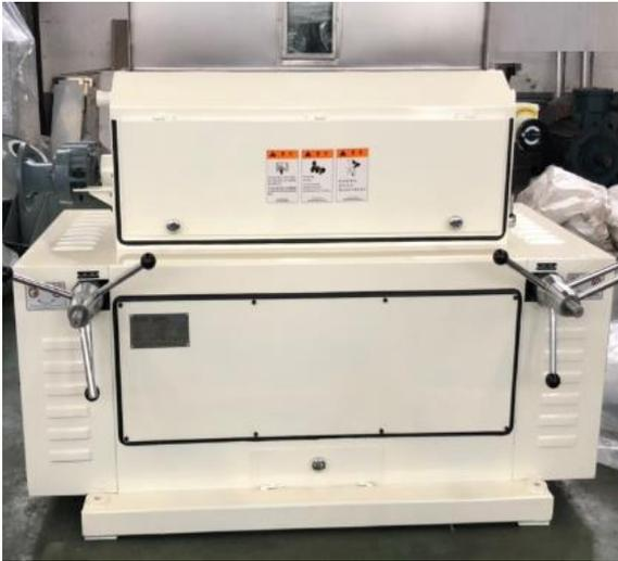
Cereal milling roller mill with 1000mm L x 300mm diameter rolls with fluting suited to kibble production.
