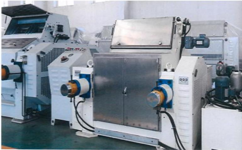
Heavy duty flaking mill fitted with 1250mm L x 600mm diameter rolls for breakfast cereal flaking installation.
