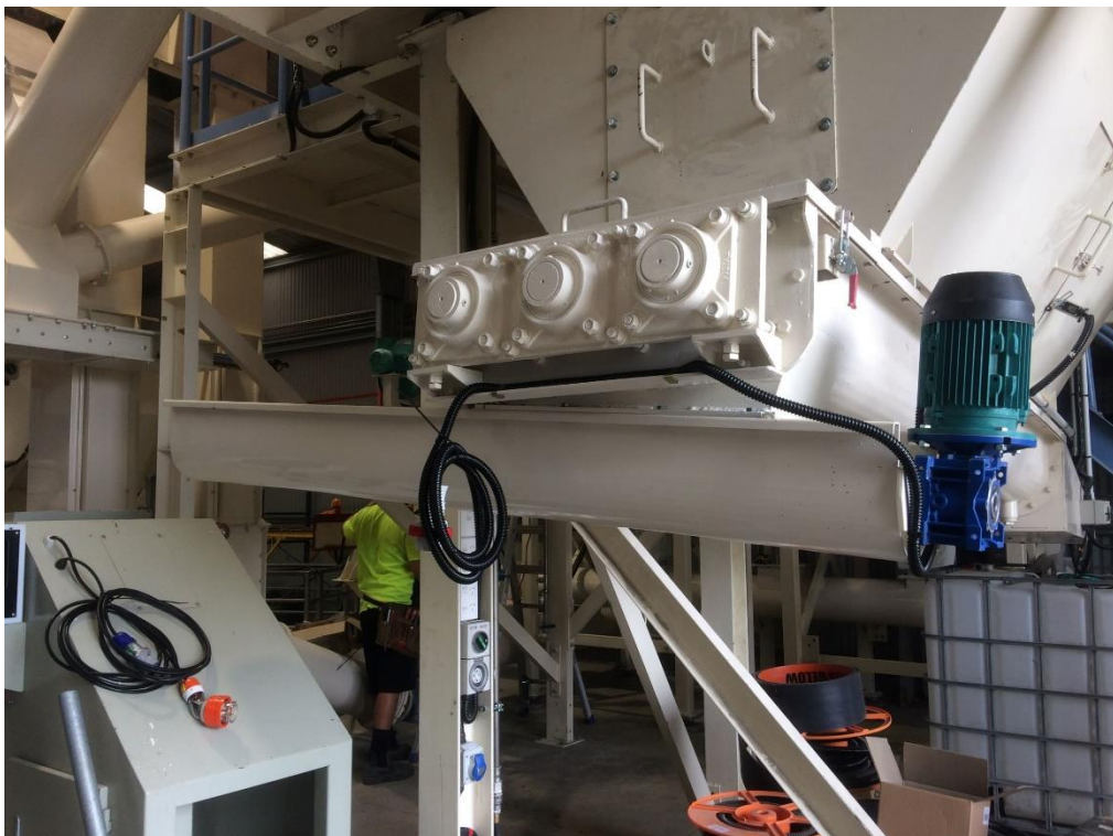
Metering dischargers with variable speed control feeding packing machine
